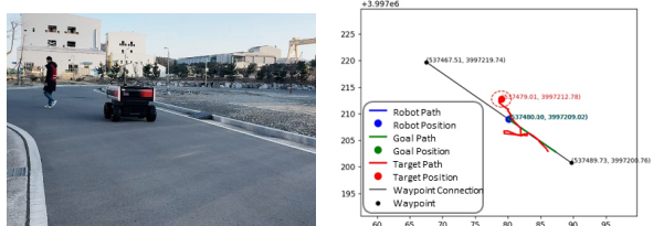
(d) Target object deviates to the left from the designated path
