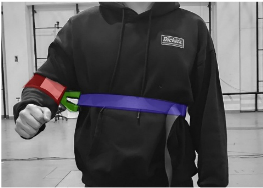
[Fig. 10] Limiting shoulder range of motion with straps to mimic frozen shoulder conditions
