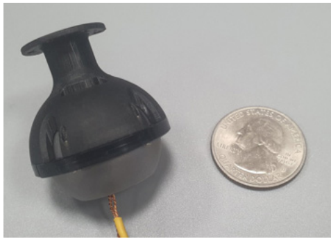
[Fig. 1] Functional prototype of the variable-stiffness ball-socket joint using electropermanent magnet actuator embedded
