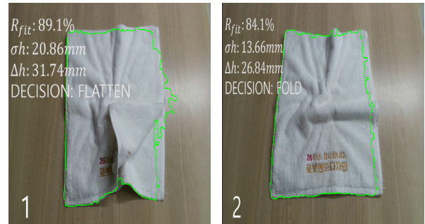
[Fig. 7] The TTCC model evaluates towel geometry from the RGB-D camera and determines the task based on tunable thresholds ( R_{fit} > 0.77 , \sigma_h < 15 mm, \Delta h < 30 mm). When all criteria are satisfied, the towel is classified as FOLD; otherwise, FLATTEN
