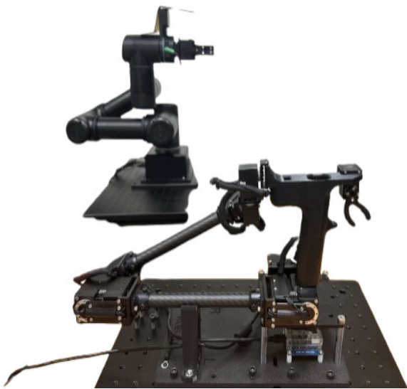
[Fig. 2] Teleoperation tool used for collecting human demonstration data
