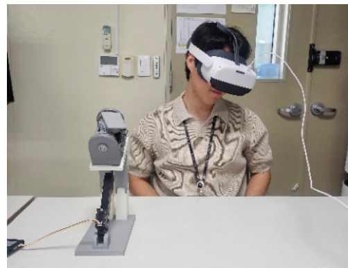
[Fig. 11] Teleoperation experiment of HMD-based head motion
