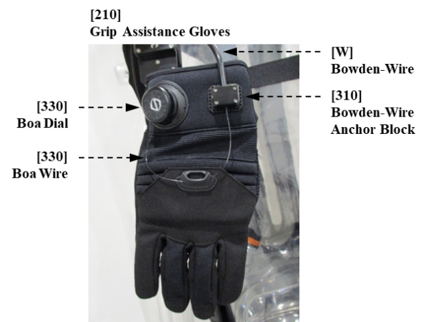
[Fig. 5] Grip Assistance Gloves Components (Adapted from Korean Patent No. 10-2760331) [12]
