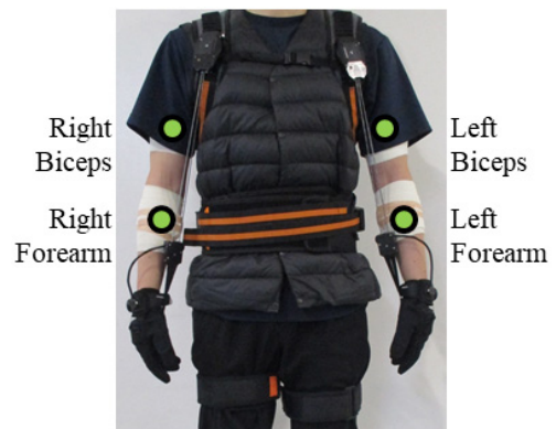
[Fig. 8] Attachment locations of EMG sensors on the body
