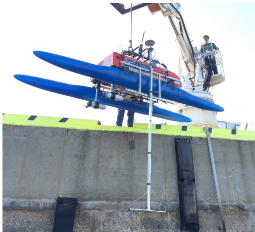
[Fig. 5] Unmanned surface vehicle equipped with acoustic positioning system
