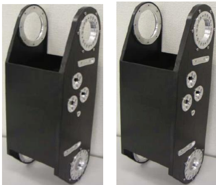
Fig. 7. CFRP frame with high strength and light weight
