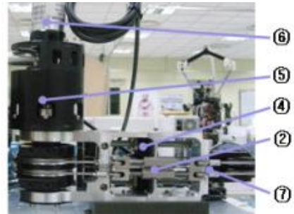
Fig. 3. Cable Ball-Screw module (Reduction ratio1/104)
